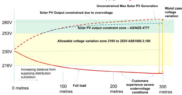
Figure A4.5 -LV Feeder Voltage Profile with Solar PV and Reduced Distribution Supply Voltage
