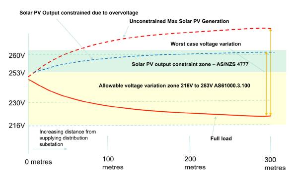
Figure A4.4 - LV Feeder Voltage Profile with Solar PV
